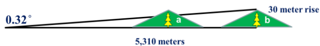
Figure 1. Schematic of vertical definition. In this illustration, a promontory (green) the height of a tree (yellow) is considered flat if it occurs at 5,310 m. distance (b) and not flat if it occurs at any closer distance (a).
